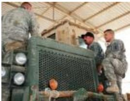
Mike Rone, a TACOM Life Cycle Management Command Engineer logistics assistance representative assigned to 402<sup>nd</sup> Army Field Support Brigade, advises Soldiers from the 561<sup>st</sup> Engineer Company during repairs to a Caterpillar 621B Scraper at Joint Base Balad, Iraq. Working together, they managed to repair rather than replace the engine. (Photo by Summer Barkley).
